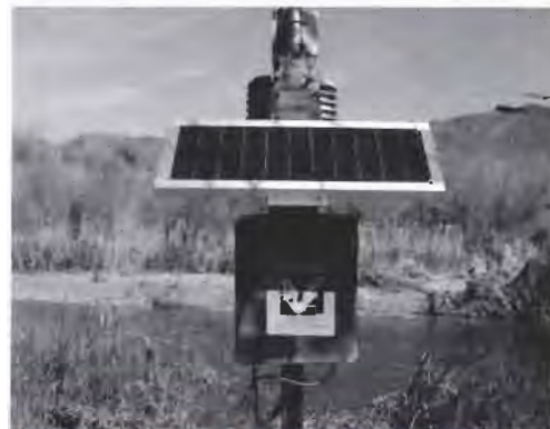
Monitoring stations like this one are posted along the Las Vegas Wash to record bat calls and migratory patterns.
