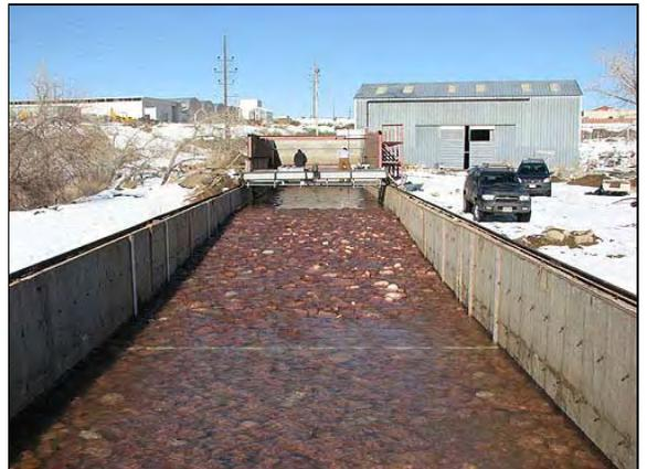
CSU's outdoor flume for testing stabilization weirs
