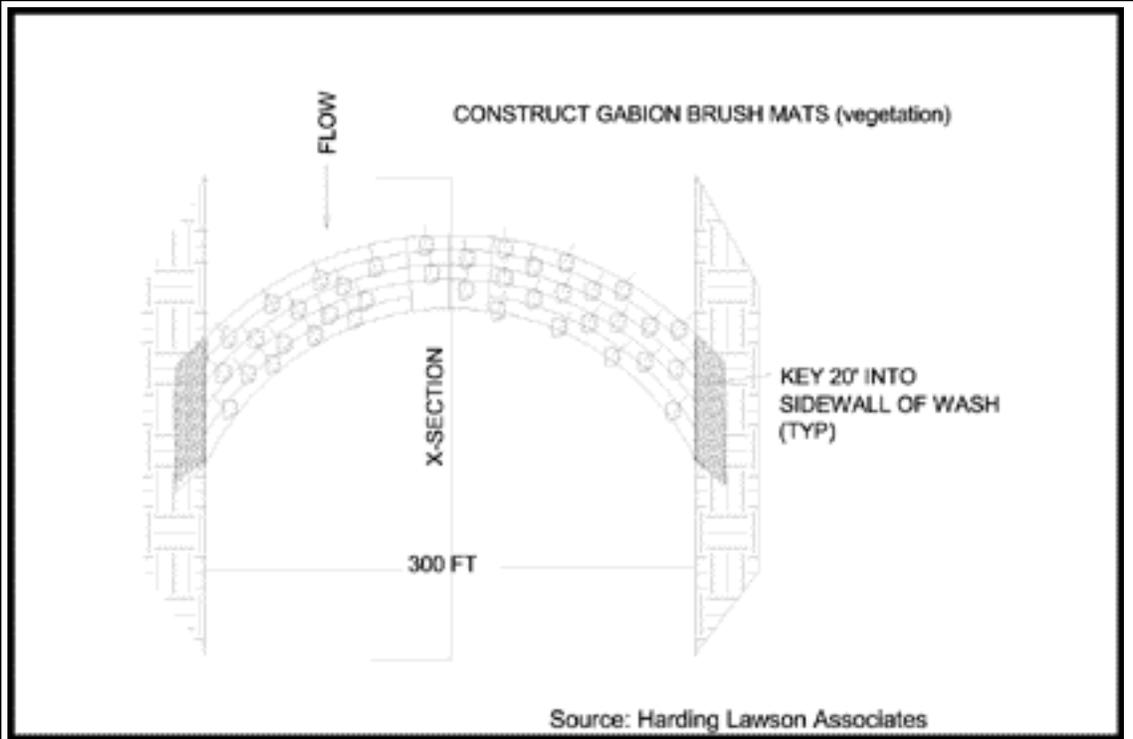
Figure E – Plan view of prototype erosion control structure.
