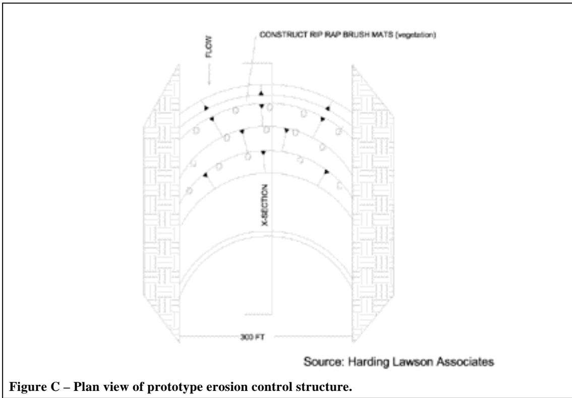
Figure C – Plan view of prototype erosion control structure.
