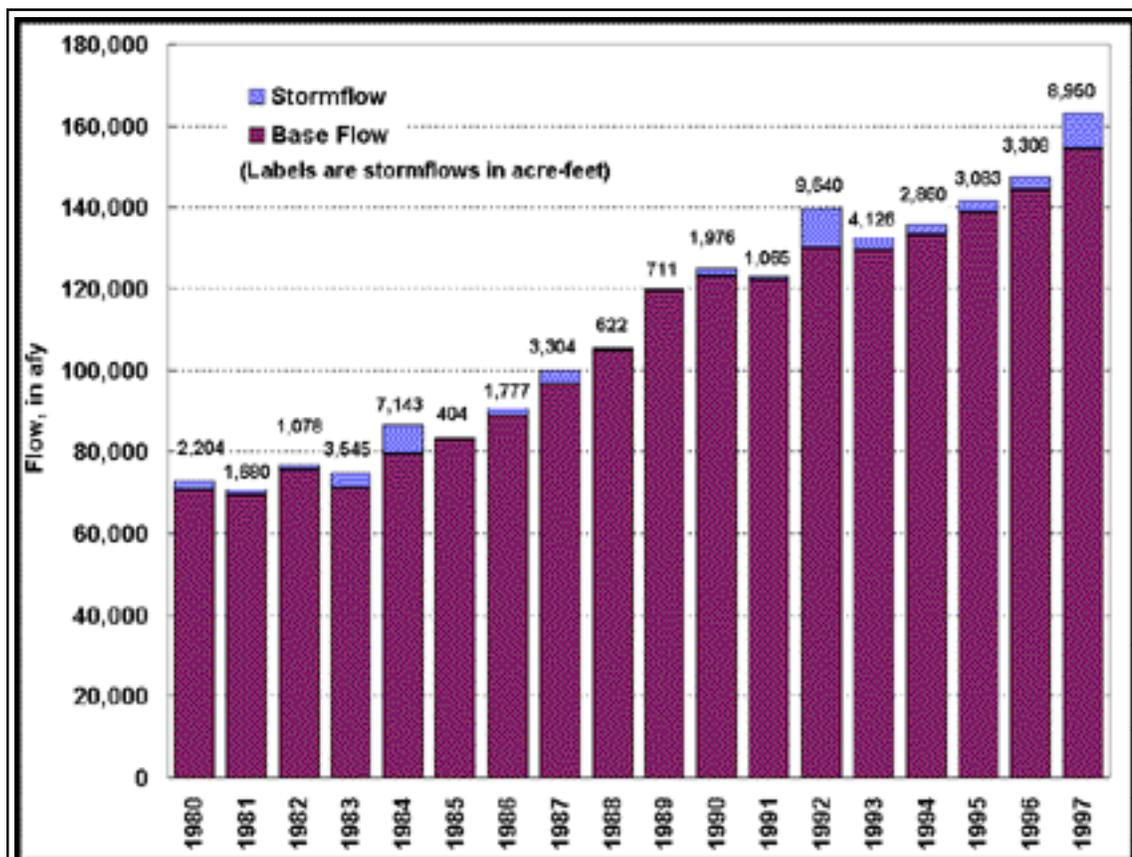
Figure 2.9 – Annual stormwater flow and base flow in lower Las Vegas Wash, estimated using daily mean flows (Method 2).
