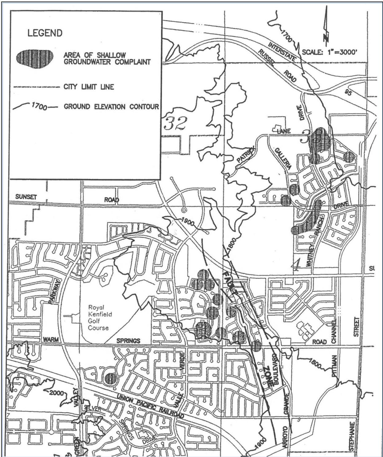
Figure 2. A map showing areas of concerns with near-surface groundwater (modified from SEA, 1994)
