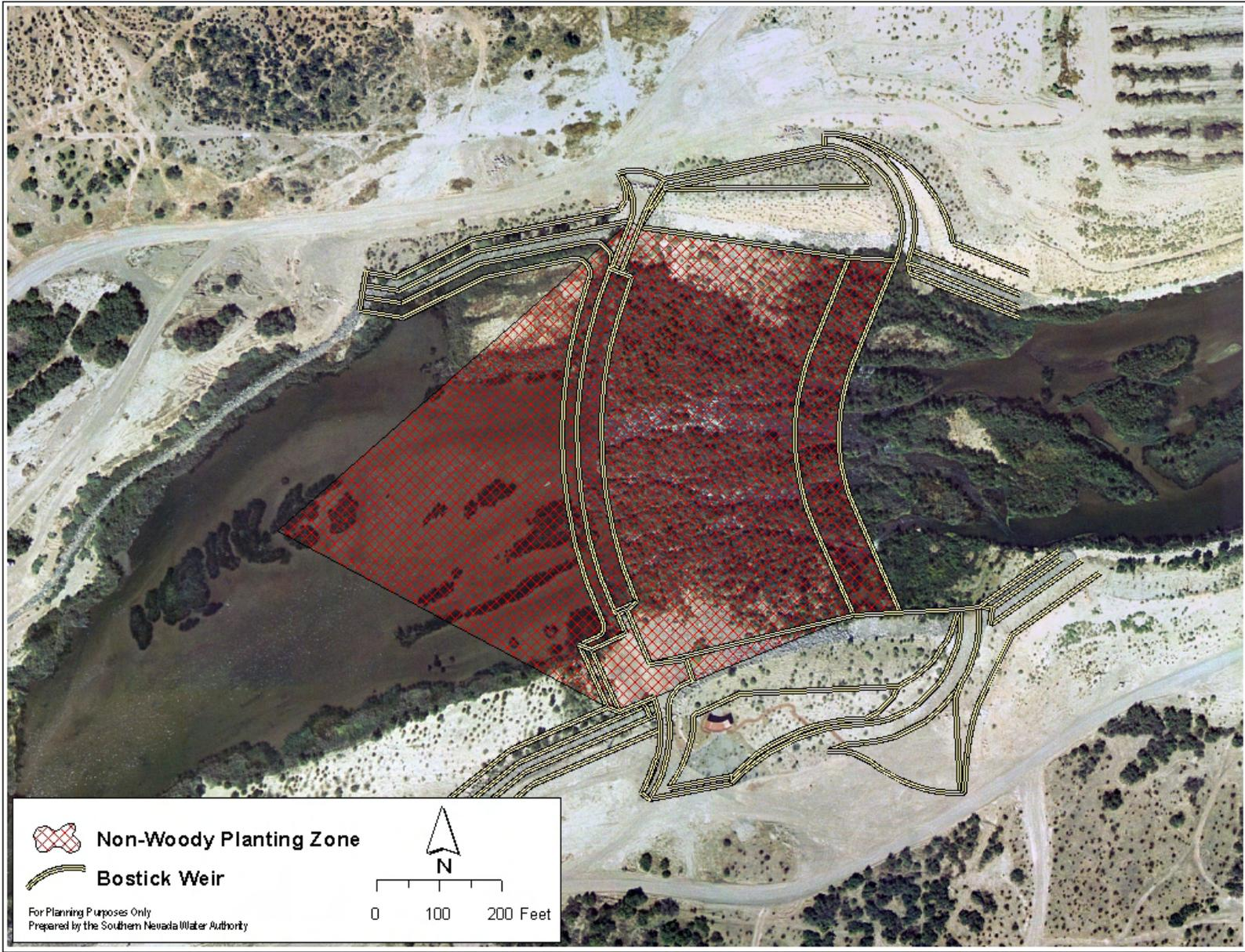
Figure 6: Locations on and near erosion control structures where woody species should not be planted.
